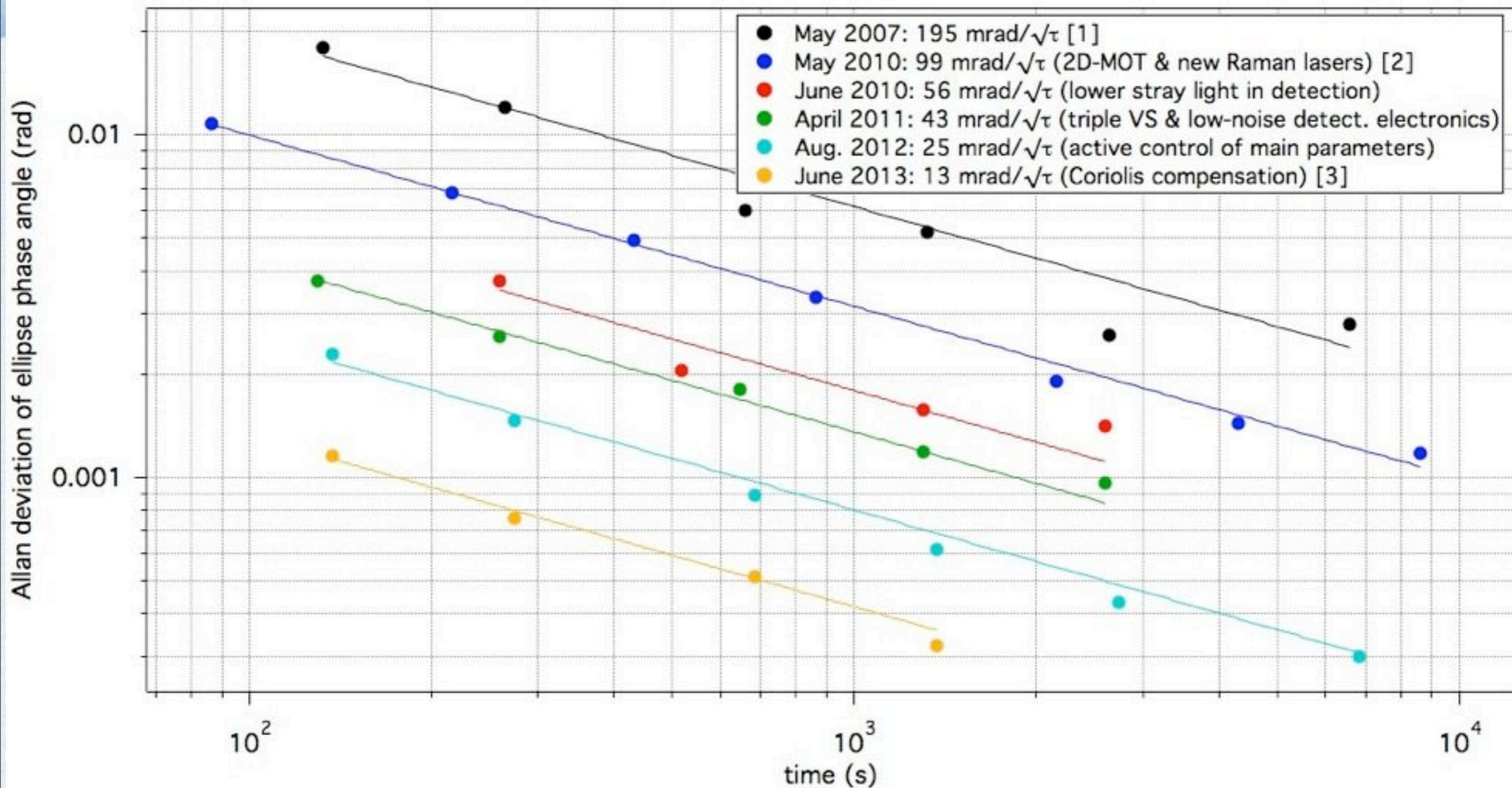
**Current sensitivity to differential acceleration:  $3 \times 10^{-9}$  g @ 1s (=QPN for  $4 \times 10^5$  atoms)**
