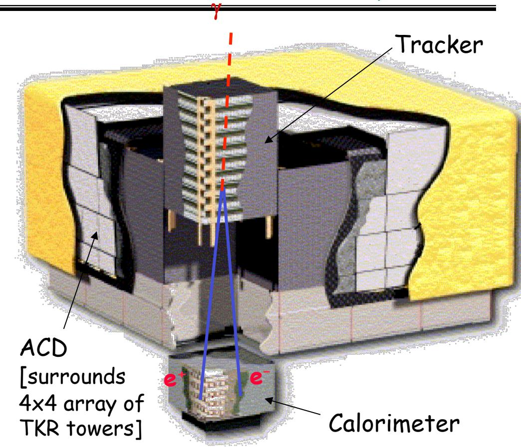
Systems work together to identify and measure the flux of cosmic gamma rays with energy 20 MeV -  $>300$  GeV.
