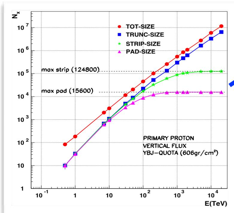
4 different gain scales used to cover a wide range in particle density:
