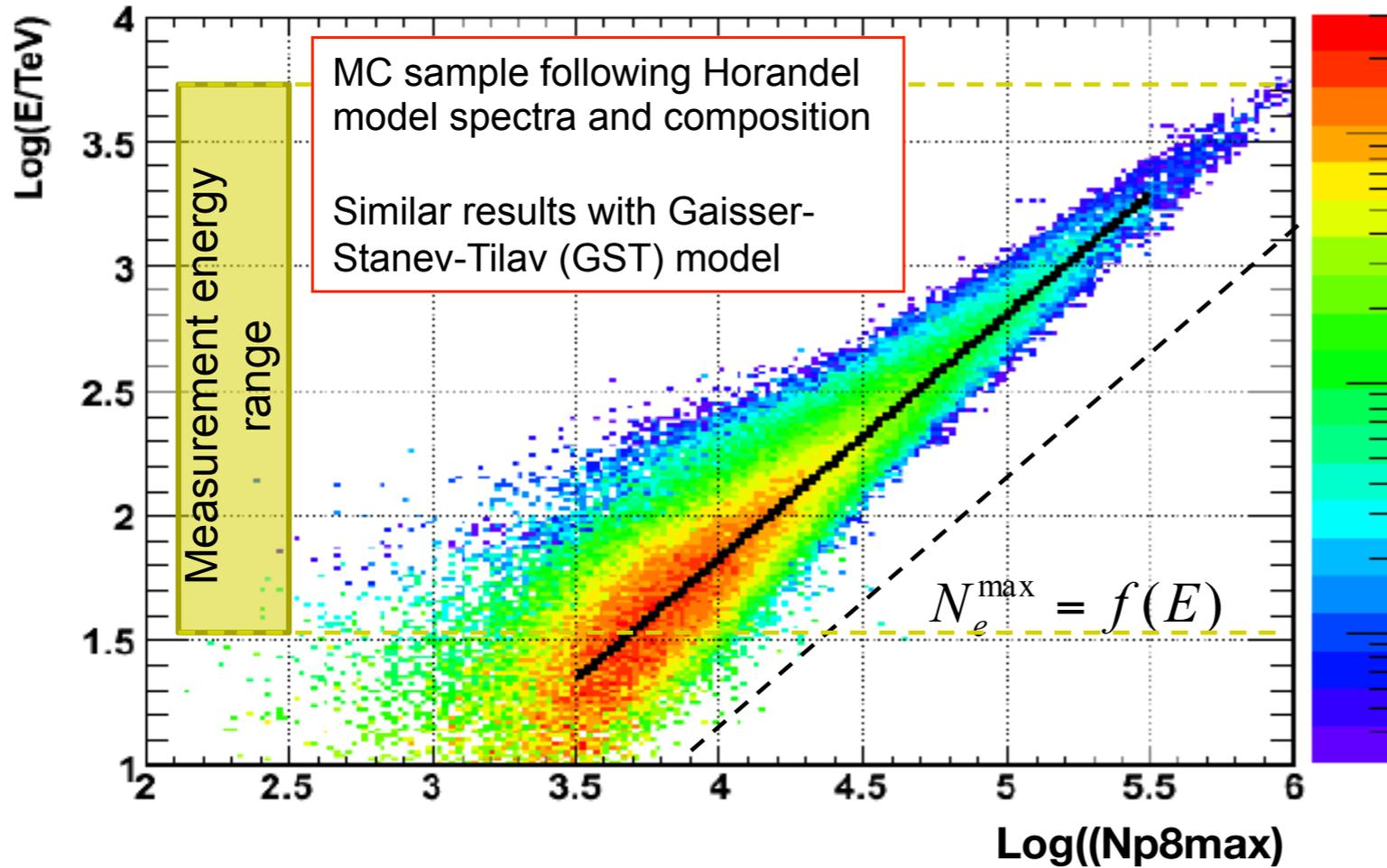
The measurement of Np8 and the (age correlated) LDF slope allows estimating the truncated size at the shower maximum.
