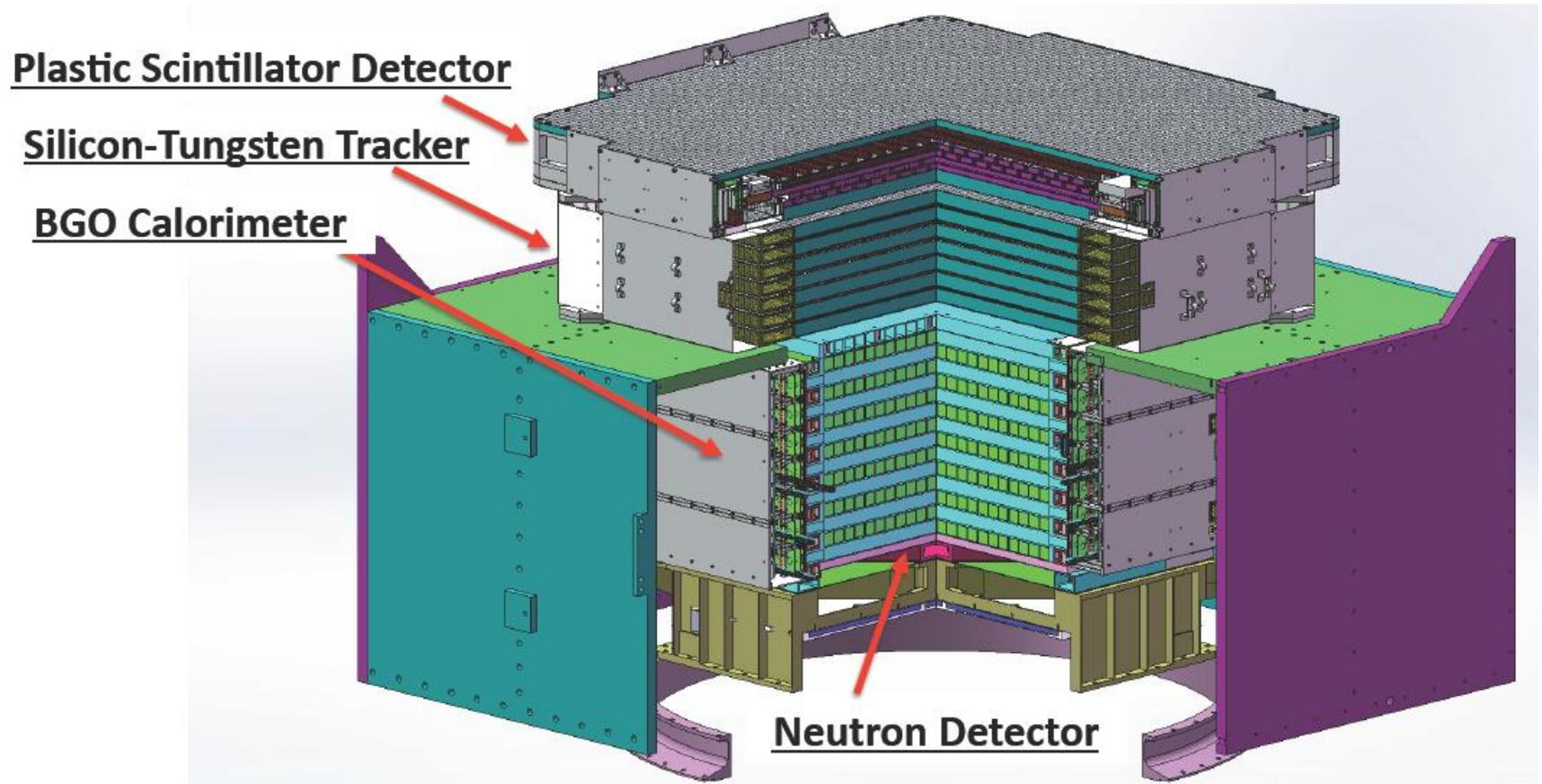
W converter + thick calorimeter (total  $33 X_0$ )
