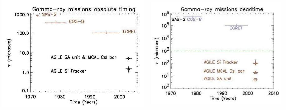
AGILE fast timing allows, for the first time, a search for sub-millisecond transients in the  $\gamma$ -ray energy range.
