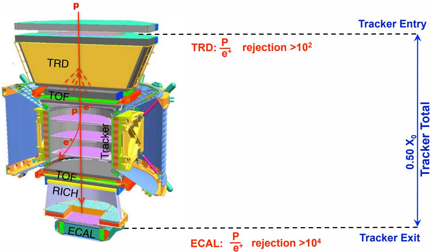
a) Minimal material in the TRD and TOF
