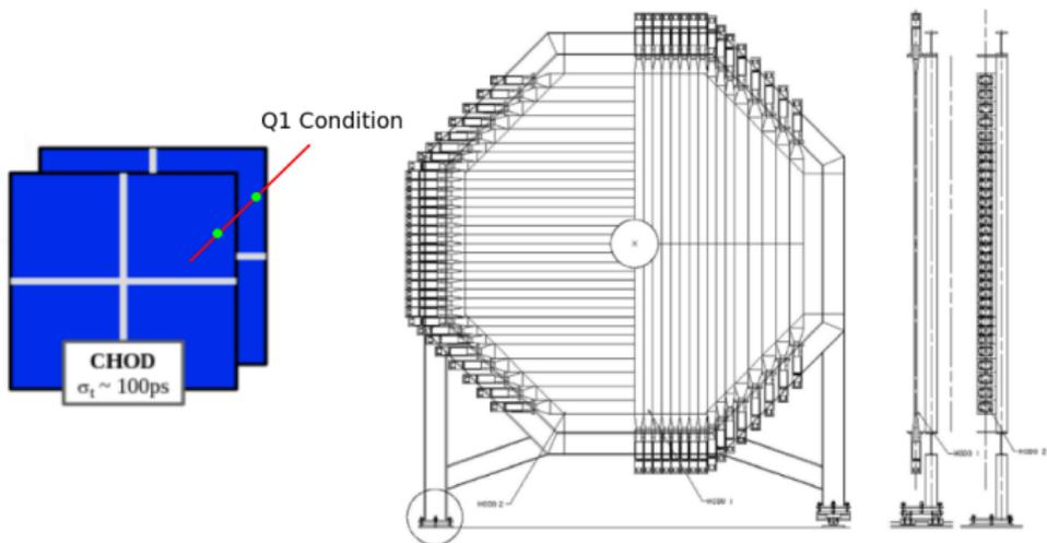
Coincidence of hits in the same quadrant in the front and back planes is the Q1 condition
