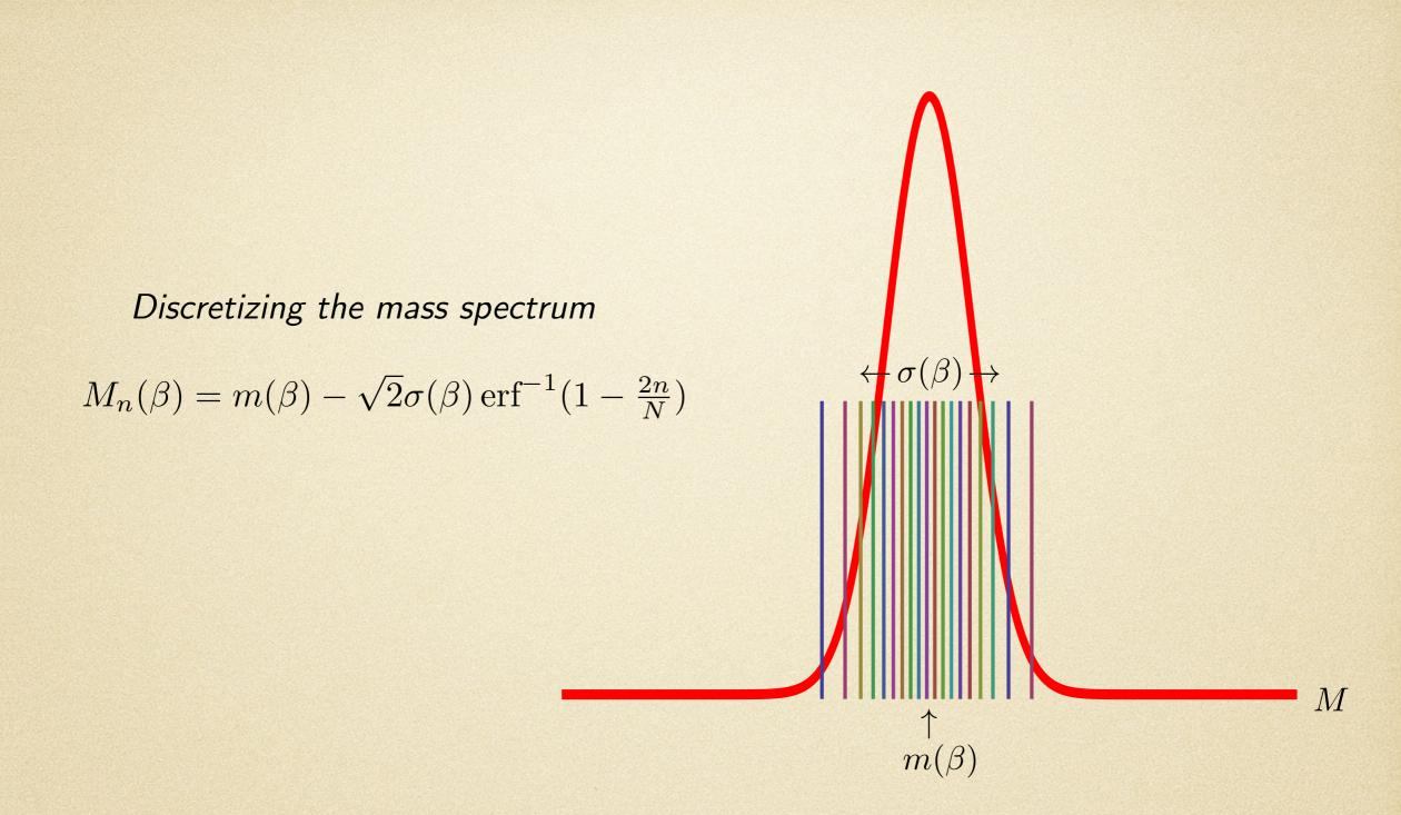
The mass distribution is divided into N equal probability sections, each of these wide sections is represented by a (temperature dependent) thin mass level.
