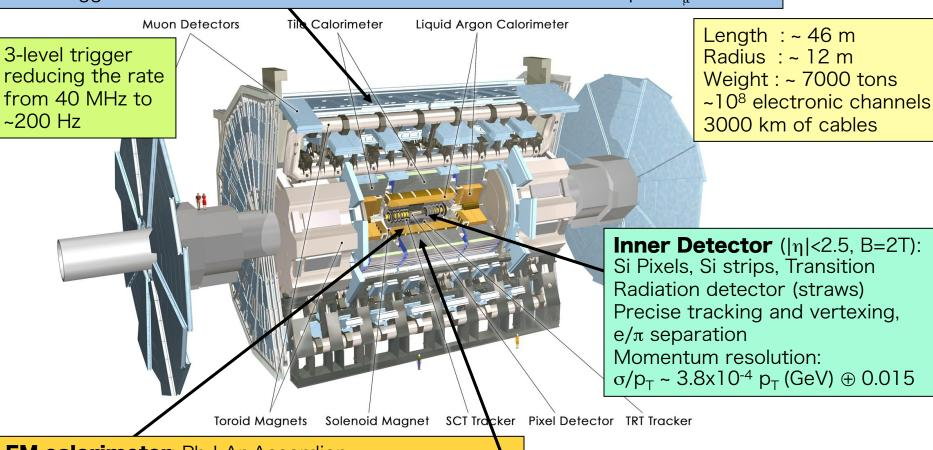
**EM calorimeter**: Pb-LAr Accordion  $e/\gamma$  trigger, identification and measurement E-resolution:  $\sigma/E \sim 10\%/\sqrt{E}$
