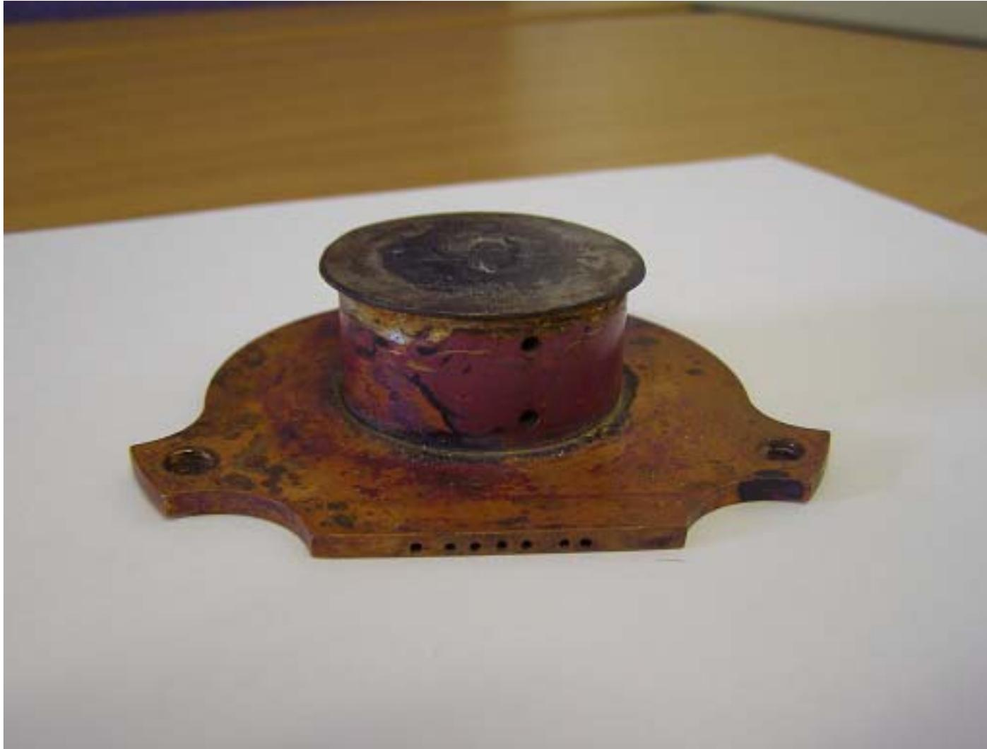
Target blank with copper boss and steel plate.
