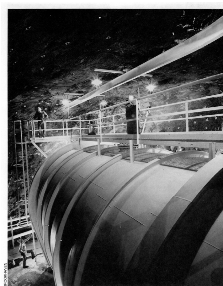
Davis' neutrino detection apparatus one kilometer underground in the Homestake Gold Mine, Lead, South Dakota. The tank contains 400,000 liters of perchloroethylene.
