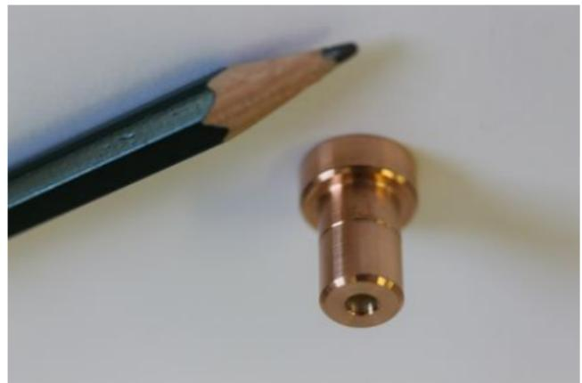
Additional copper is removed to achieve the final outer shape of the Laval nozzle.
