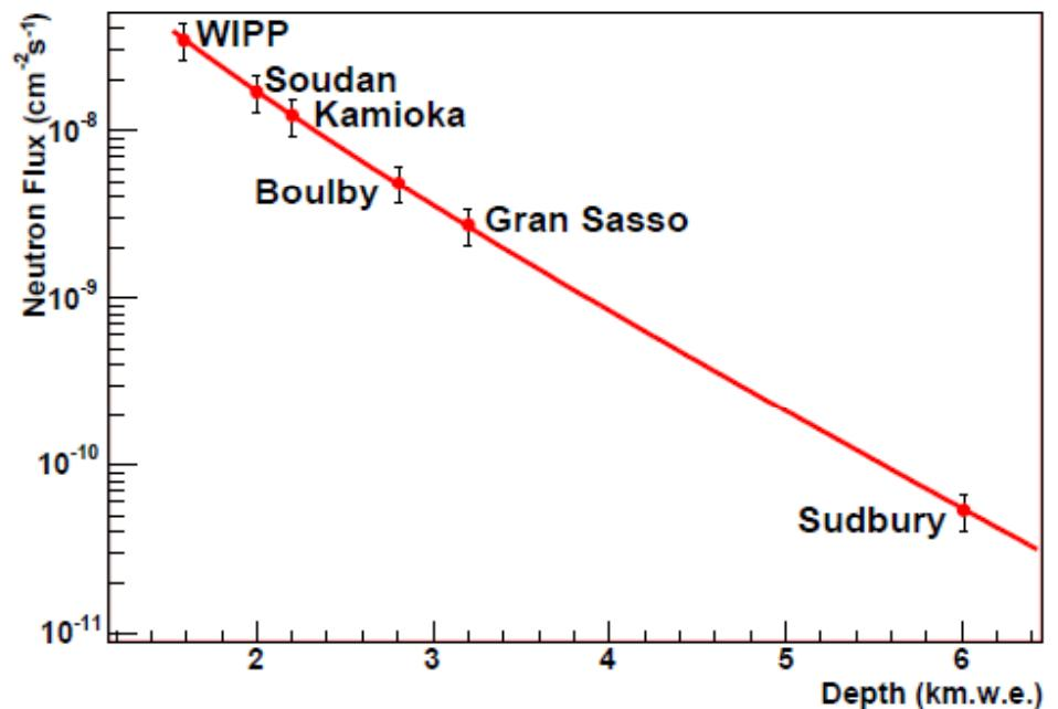
FIG. 14: The total muon-induced neutron flux deduced for the various underground sites displayed. Uncertainties on
