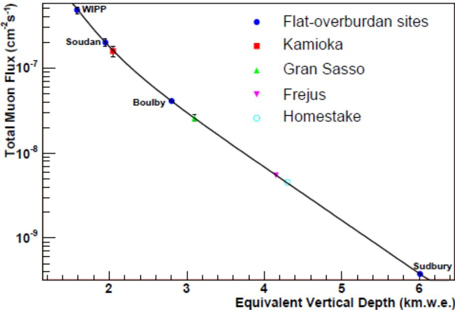
FIG. 3: The total muon flux measured for the various underground sites summarized in Table I as a function of the equivalent vertical depth relative to a flat overburden. The
