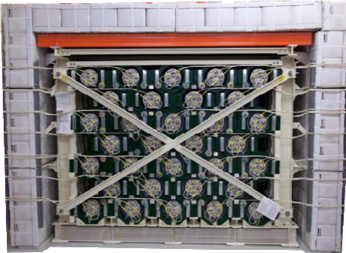
HALO is using lead blocks from a decommissioned cosmic ray monitoring station
