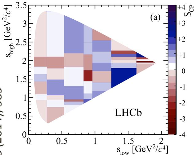
$$S_{CP}^i \equiv \frac{N_i^+ - \alpha N_i^-}{\sqrt{\alpha(N_i^+ + N_i^-)}}, \quad \alpha \equiv \frac{N^+}{N^-}$$
