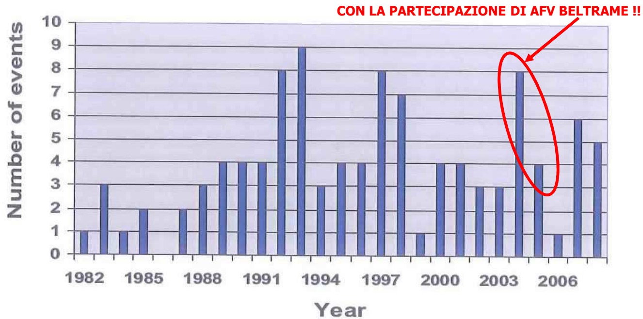
Reported accidental meltings of radioactive sources (80% in steel)
