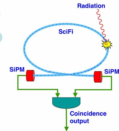
*a mesh of scintillating fibers read-out at both ends by means of Silicon PhotoMultipliers (SiPM)*
