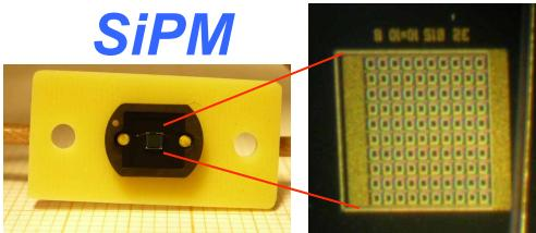
*the SiPM can detect the very short scintillation light pulse produced by gamma interaction*
