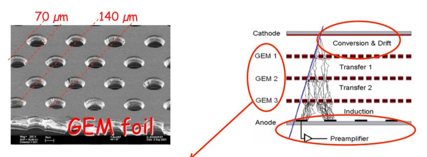
Working with different levels of gain it is possible to obtain high level of gamma-neutron discrimination
