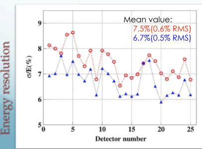
$\sigma/E$  @ 59.5 keV for each detector with new PMTs with higher quantum efficiency (blu points) and with previous PMT EMI-Electron Tube (red points).
