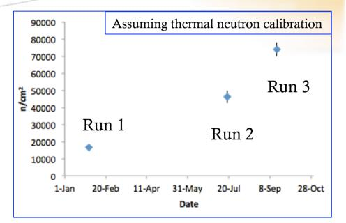
Slope between Run2/3 ≈ 460 n/cm<sup>2</sup>/day Naked CR-39 detectors show same behavior High energy background Cfr cosmic rays≈ 850 particles/cm<sup>2</sup>/day
