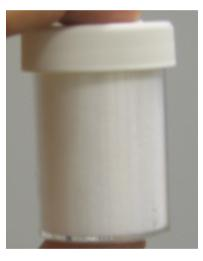
**TEST:** no signal observed at ENEA-IMRI thermal neutron source **CONCLUSION**: The detector used by Cirillo et al are sensitive to fast neutrons
