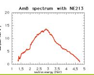
The AmB spectrum after traversing water gets moderated to epithermal+ thermal → Partially moderated (PM) spectrum
