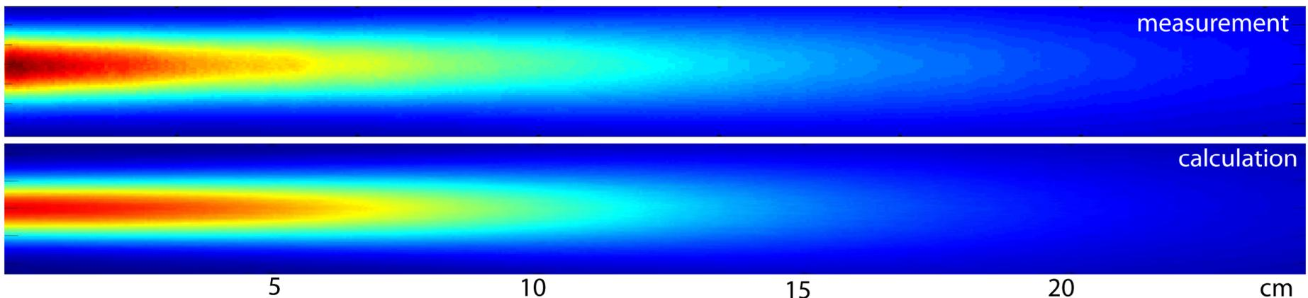
Differences between measurements and calculations due a misalignment: the Gafchromic films were not well aligned with the central axis of the electron beam.
