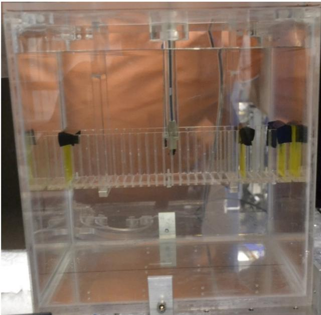
Ionization chamber experiment: ion chambers are well-established detectors for conventional radiotherapy beams (where field size is of the order of 5-10 cm, energy up to 25 MeV, ms bunch duration and kHz repetition rate) but their response at higher energy and shorter beams is still unknown.
