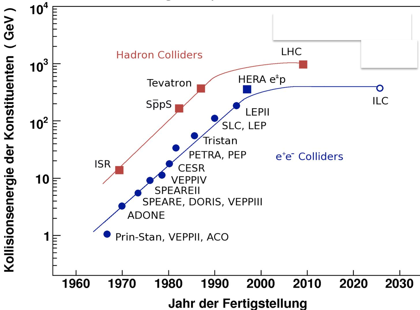
Practical limit for accelerators at the energy frontier: Project size and cost increasing with the energy ! New technology needed...
