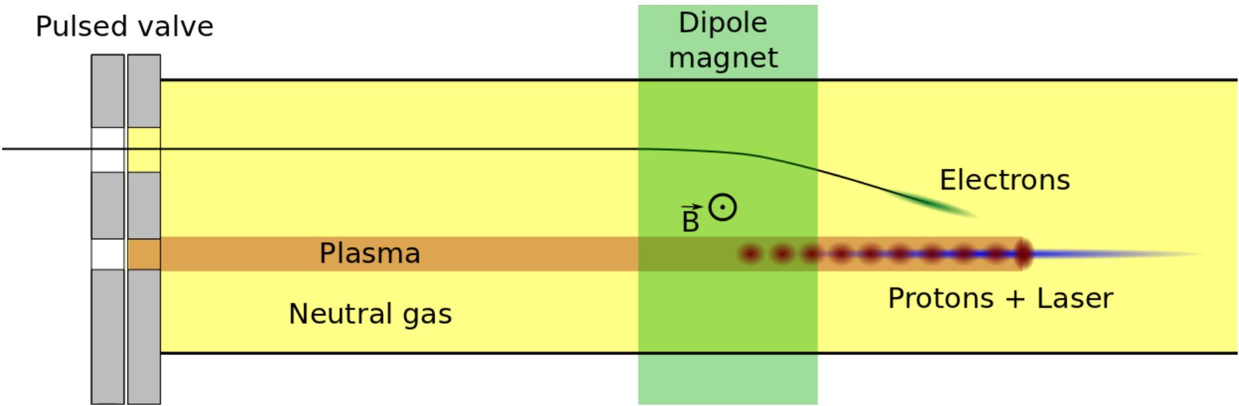
Electron bunch injected off-axis at an angle, so that it merges with the proton bunch once the modulation is developed and the phase velocity is high.
