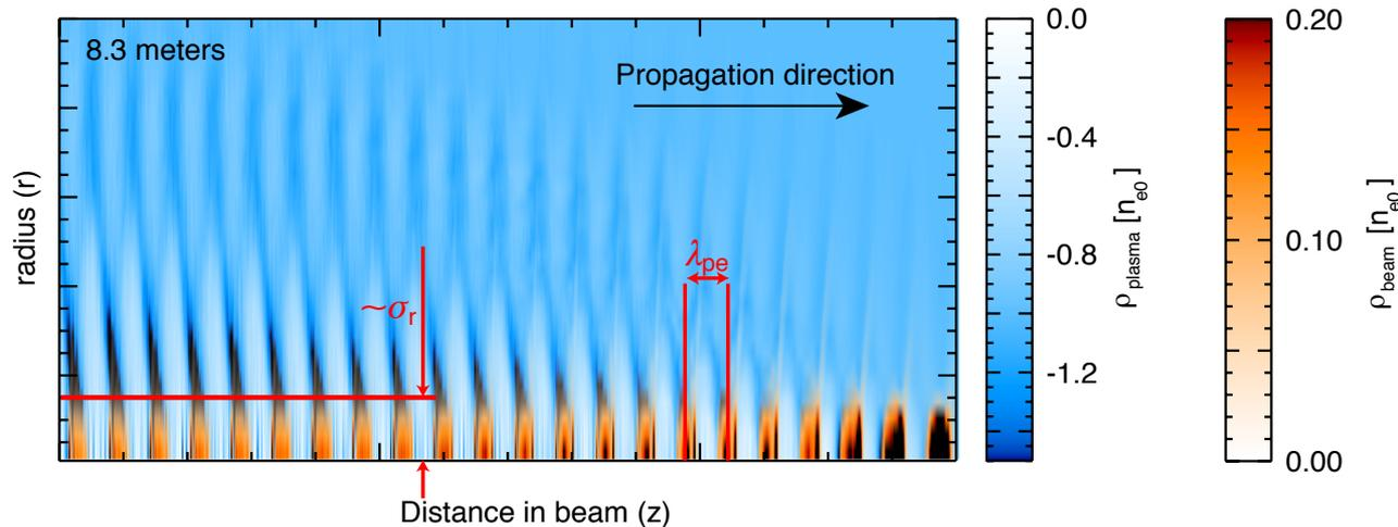
Microbunches are generated by a transverse modulation of the bunch density (transverse two-stream instability). Naturally spaced at the plasma wavelength, and resonantly drive wakefields to large amplitudes. (N. Kumar, A. Pukhov, and K. V. Lotov, Phys. Rev. Lett. **104**, 255003 (2010)).
