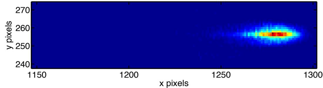
Simulation of scintillator screen shot from full simulation of electrons in plasma cell & tracking through spectrometer
