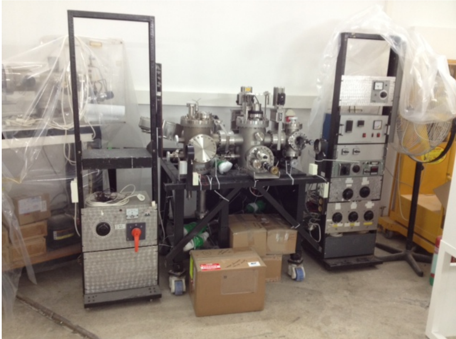
Shipment contents: 3-chamber deposition and transfer setup mounted on a metal stand, 2 electronic racks, 4 boxes with spare parts and documentation
