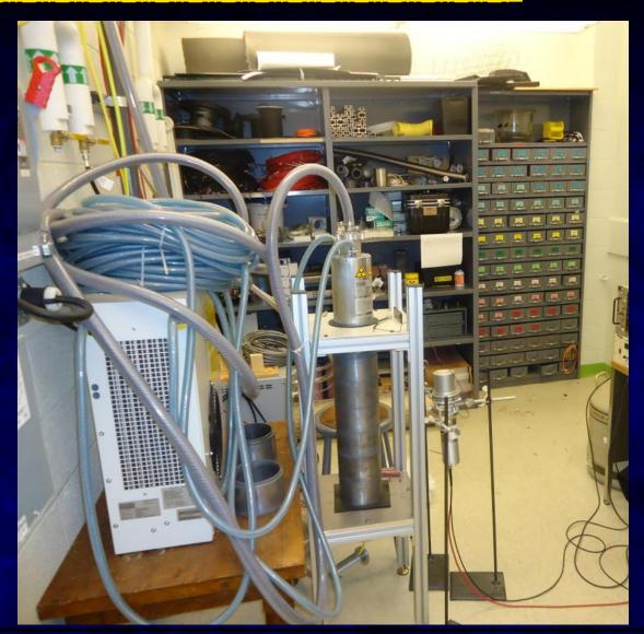
NSD-35-DD-C-W-S custom-built for low flux  $(\sim 1n/s - \sim 10^5 n/s)$  and water tightness
