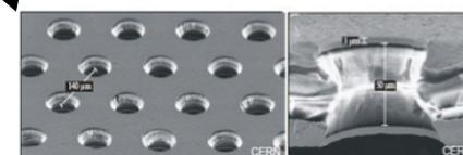
Electron microscope photograph of a GEM foil
