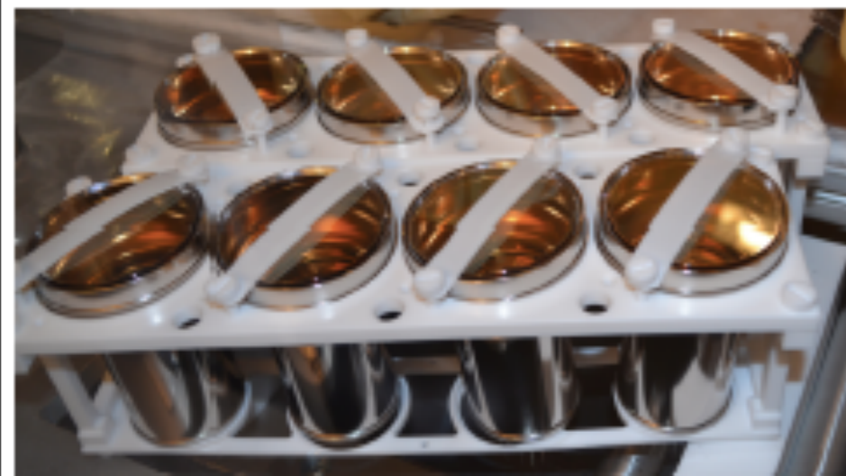
PMT mounted in low radioactive holders
