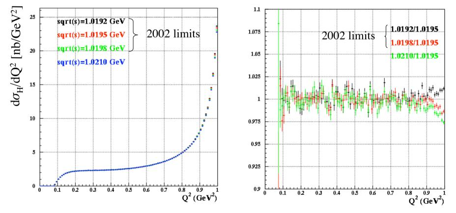
No big deviation found below 0.90 GeV<sup>2</sup>. In the ratio, the radiator should cancel. Cross check with muon data/MC comparison.
