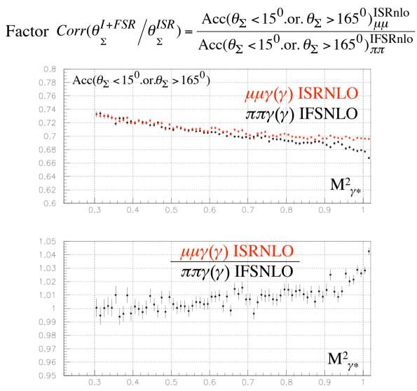
~1% correction for the ratio - ~70% correction for absolute measurements
