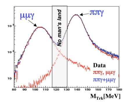
$\begin{pmatrix} M_{\text{Trk}} \text{ obtained from solving} \\ \left( M_{\phi} - \sqrt{\vec{p}_{1}^{2} + M_{trk}^{2}} - \sqrt{\vec{p}_{2}^{2} + M_{trk}^{2}} \right)^{2} - (\vec{p}_{1} + \vec{p}_{2})^{2} = q_{\gamma}^{2} = 0$
