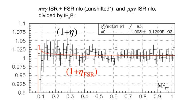
Dividing for  $(1+\eta_{FSR})$  and fitting with P0 gives A0 = (1.000 ±0.128E-02). Radiator H cancels, leaving only effects from (pionic) FSR.
