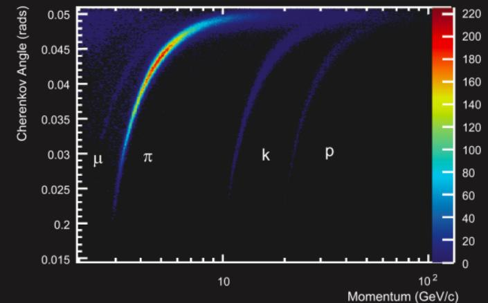
Reconstructed Cherenkov angle as a function of track momentum in the  $C_4F_{10}$  radiator. Whilst the RICH detectors are primarily used for hadron identification, a distinct muon band can also be observed. From The LHCb RICH Collaboration: Performance of the LHCb RICH detector at the LHC
