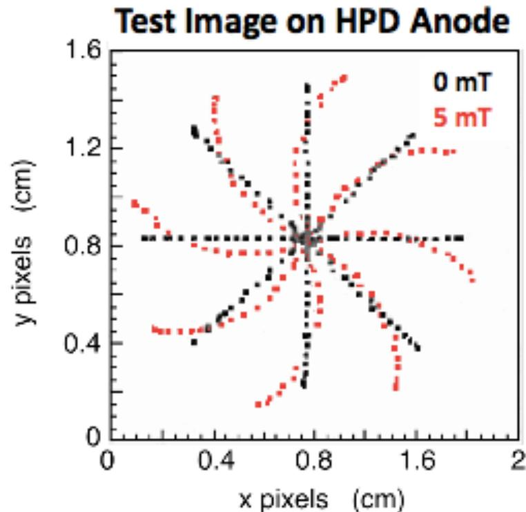
Projection of test pattern with and without magnetic field to extract correction parameters
