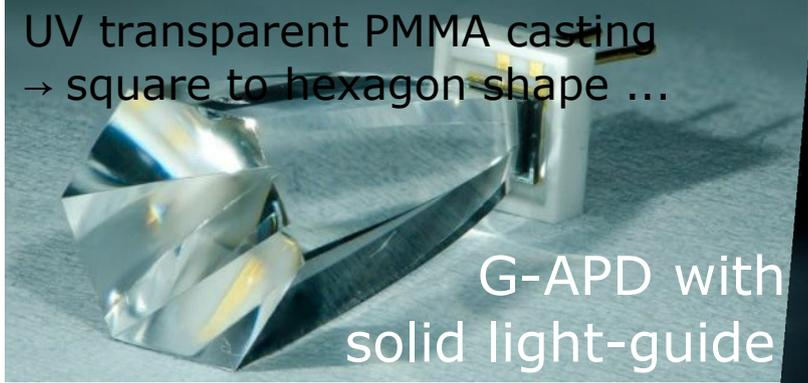
UV transparent PMMA casting
