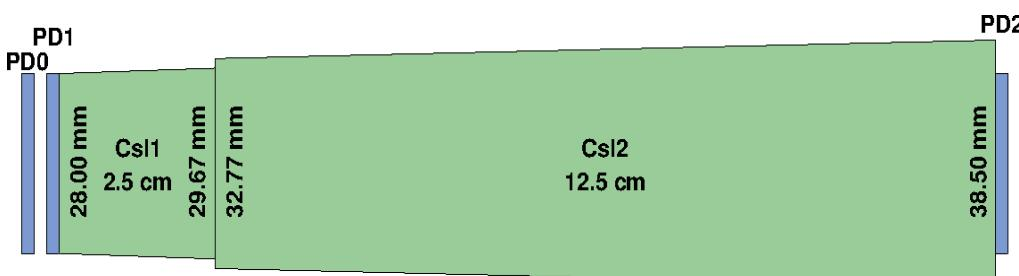
The crystals are altogether 15 cm long, what implies about 30-40% probability of secondary reactions/scatterings for particles penetrating the full length.
