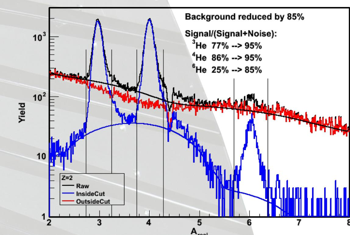
Fig. 4: Mass spectrum for  $Z=2$  particles, before (black) and after (blue) background reduction. Red histogram corresponds to the background.
