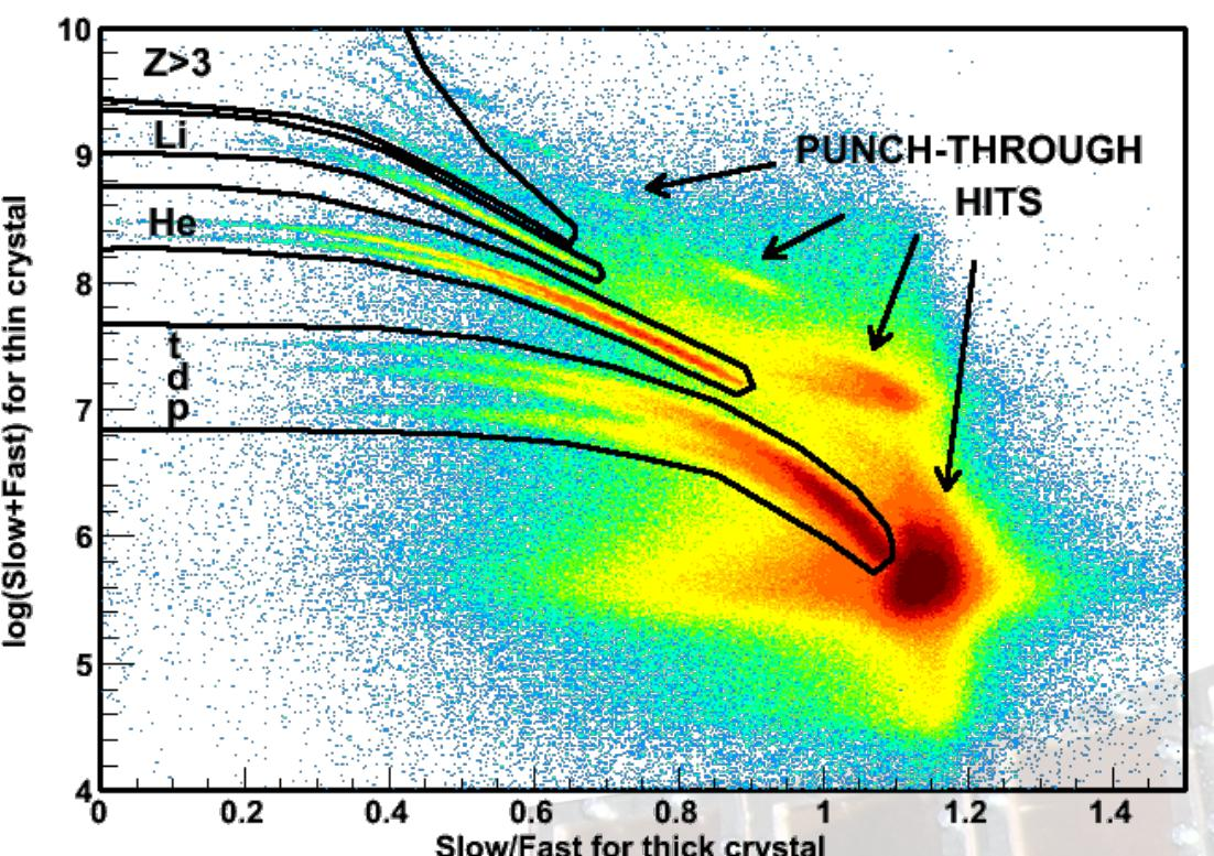
Fig. 1: Logarithm of the total light in the thin crystal vs Slow over Fast component of light in the thick crystal. The lines define borders of the regions of well identified particles (inside the cuts).
