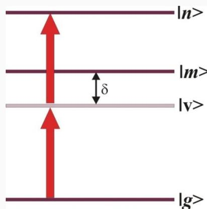
$$B(\omega) = \tau^2 \frac{|\mu_{nm}|^2 |\mu_{mg}|^2 |E|^4}{\hbar^4 (\omega_{mg} - \omega)^2}$$
