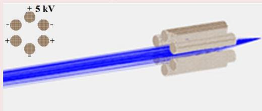
In linear regime, the hexapole provides a radial (velocity) confinement due to a quadratic potential
