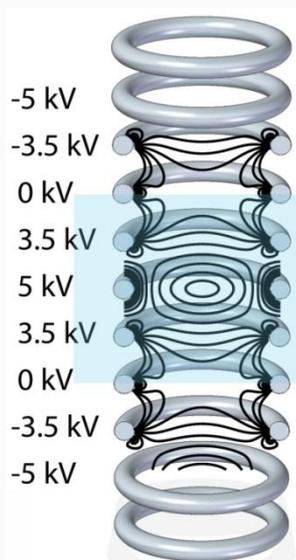
The frequency of the applied voltages determines the velocity of the moving traps. Initially, as the molecules enter the decelerator, the traps are set to move at the same speed as the molecules. Then, gradually, the oscillation frequency of the voltages is swept down resulting in the deceleration and ultimately stopping of the traps, with the molecules remaining in the traps.
