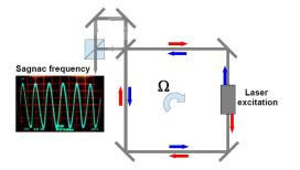
When the cavity rotates with frequency  $\Omega$ , the bit note,  $\delta f_{Sagnac}$ :
