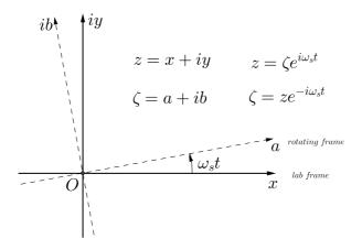
.. and if bearings noise dominates it will appear close to  $-\omega_s$  line and not to  $+\omega_s$  line  $\Rightarrow$  bearings noise can be identified and measured unambiguously...
