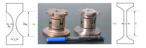
Stiffness measured in the lab, improvement by factor 5 to 10 w.r.t. old design. For the central joint (the most relevant for the differential coupling of the test masses) values for the two directions are much closer to each other. If not, the stiffer dominates resulting in lower sensitivity, & more complex dynamics (T.R.Saravanan, PhD thesis, 2013) Passive rotating 2D joint ensures good attenuation of low frequency tilt poise
