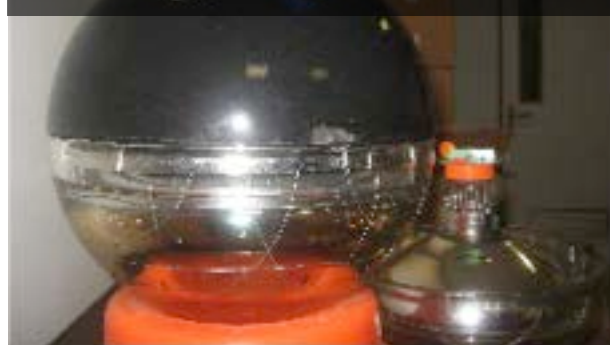
The OM: 10" Hamamatsu R7081, Front End Module, Time Calibration, LED beacons
