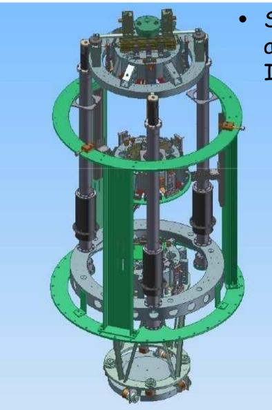
Seismic isolation improvement adding a Mechanical Filter on MC, INJ and DET suspensions
