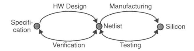
Testing is accomplished through test vectors. It verifies that internal nodes can be toggled
