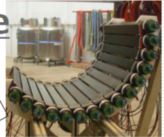
Plastic scintillator plate + SiPMs
