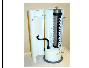
Figure 2. Model 1250 NanoMoudi 0<sup>TM</sup> (with inverted rotation)
