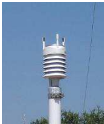
Vaisala MAWS 100/WXT520: weather station (10 min)
