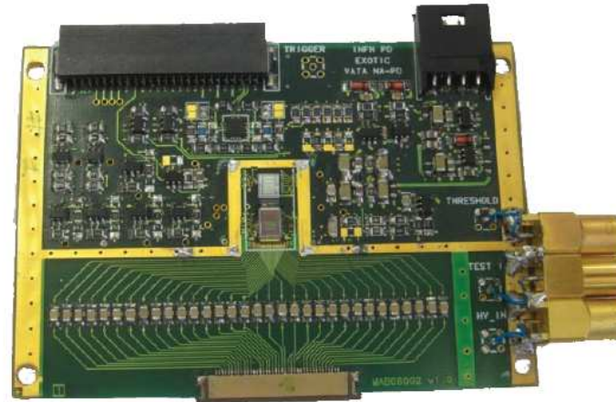
ASIC electronic board VATA
