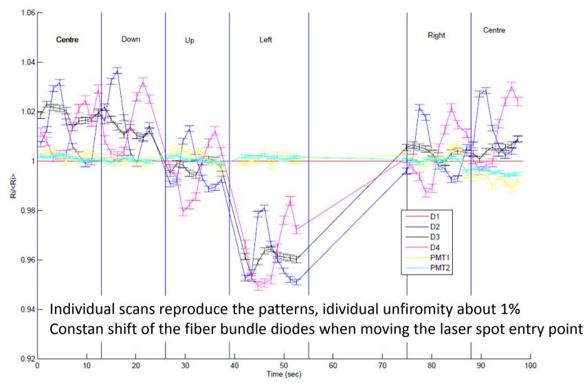
Displacements of the laser beam entry point up/down - left/right of 1 mm
