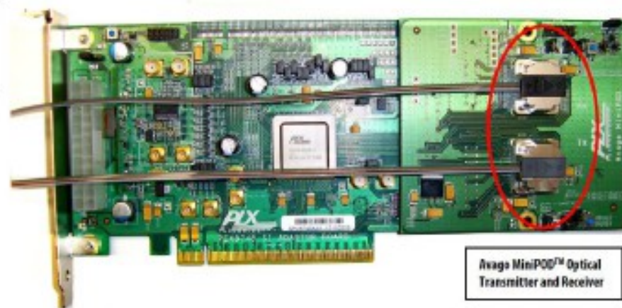
Figure 2. PEX8748 SI card with Avago Technologies MiniPOD™ adapter
