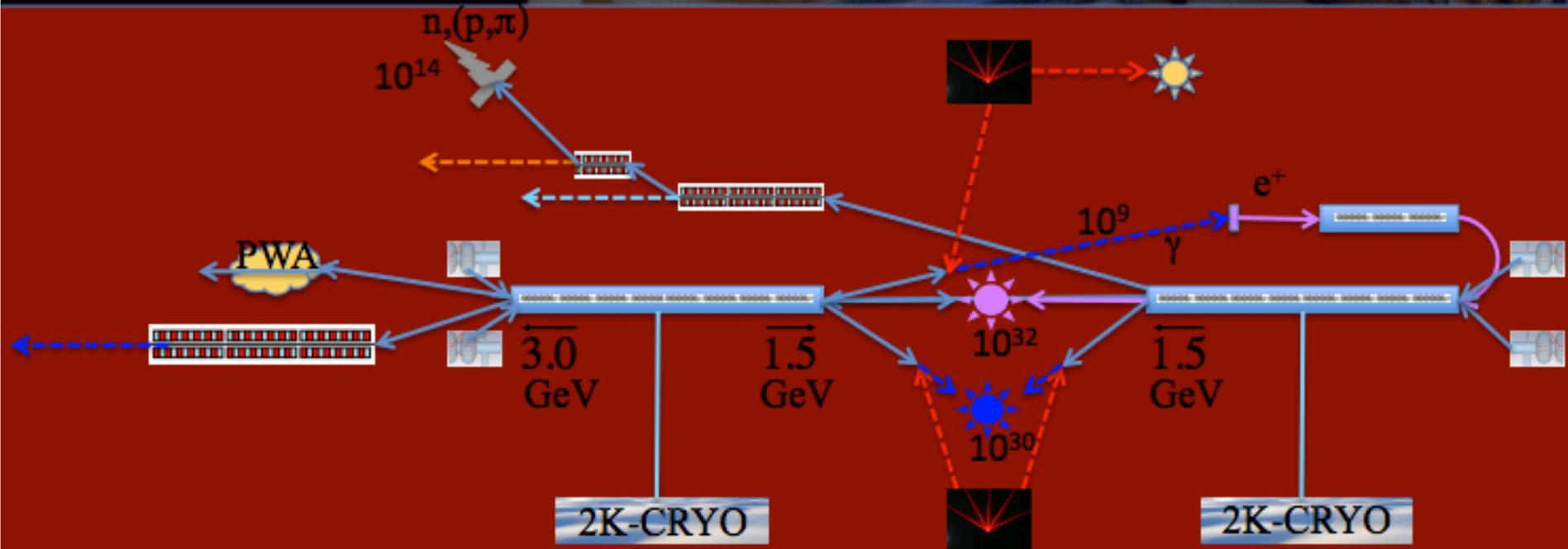
Based on a combination of a **high duty cycle radio-frequency superconducting electron linac** (SC RF LINAC) and of **high energy lasers** it will be able to produce a high flux of **electrons, photons (from infrared to  $\gamma$ -rays), neutrons, protons, pions and eventually positrons**, that will be available for a wide national and international scientific community interested to take profit of the most advanced particle and radiation sources.
