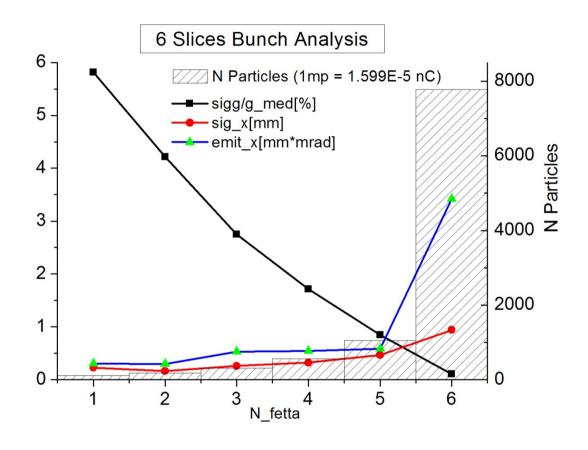
Slice N. 6 80% of the charge Q = 125 pCNormalized emittance  $\varepsilon_x = \varepsilon_y = 3.4 \text{ mm mrad}$ Relative energy spread  $\sigma_y/\gamma = 1.1\text{e-3}$
