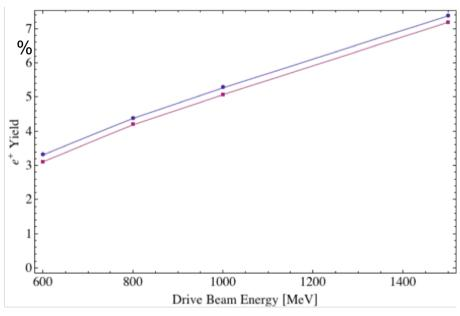
Yield of positrons within the longitudinal and transverse DR acceptance as a function of the drive beam energy for a FODO cell (red) and FDOFDO cell linac
