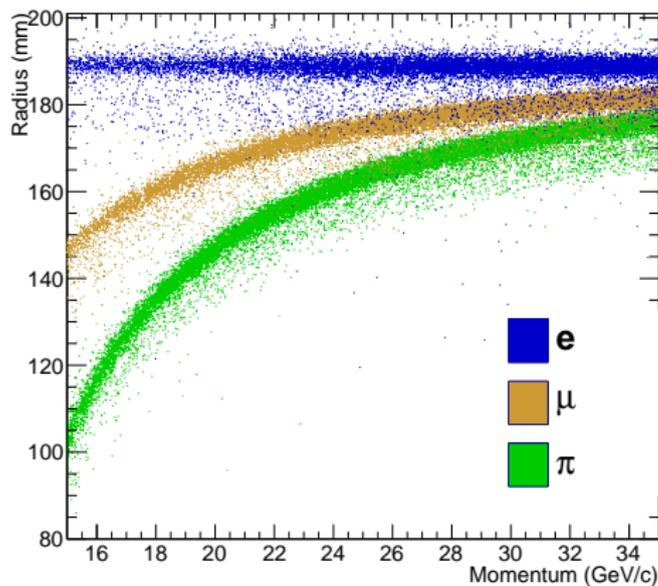
**Figure:** Reconstructed radius vs charged track momentum for  $K_{e2}$  (blue),  $K_{\mu 2}$  (brown) and signal events (green)
