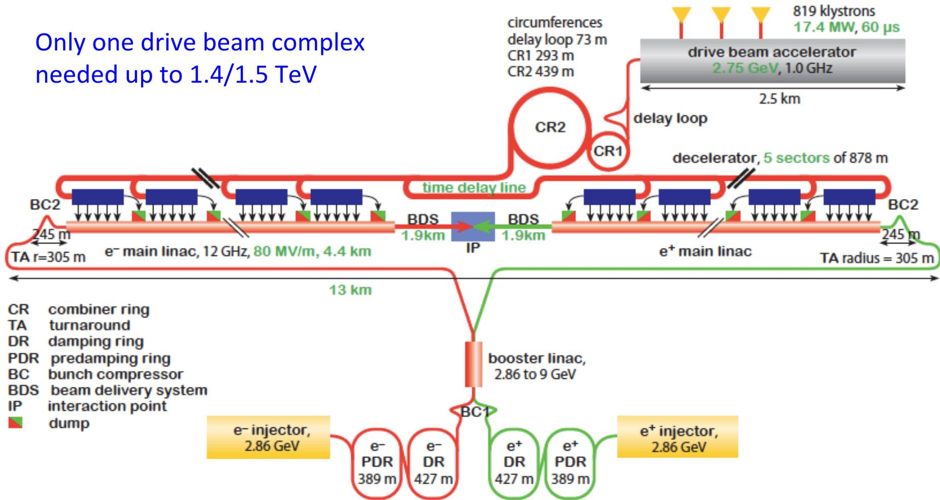
Fig. 3.2: Overview of the CLIC layout at  $\sqrt{s} = 500$  GeV. (scenario A)
