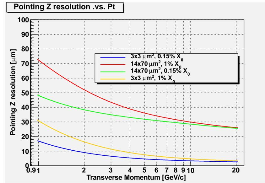
⇒ Significant improvement required wrt present LHC techno: GRANULAR ( $\phi, z$ ), THIN, LOW POWER
