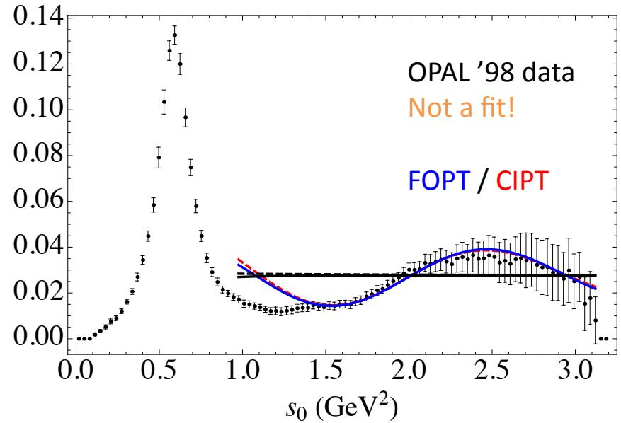
Vector channel fit with weight  $w(s) = 1$  and  $s_{\min} = 1.5$  GeV $^2$
