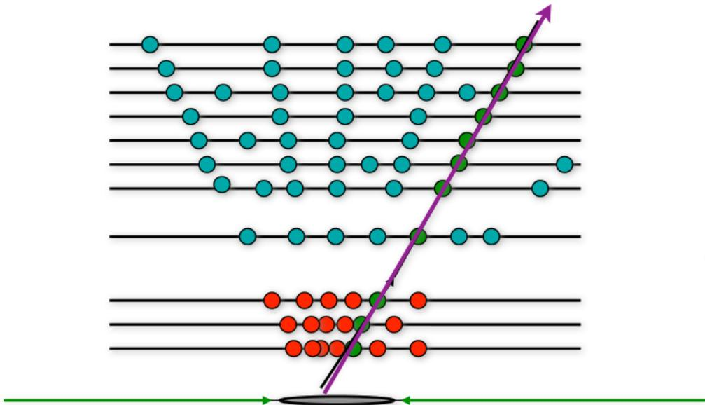
Track parameters are **re-fitted** with a Kalman Filter technique and a "*smoothing*".
