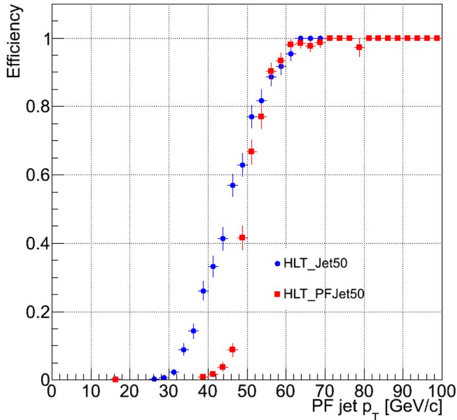
Efficiency turn-on curve (wrt offline)  $\sim 3$  times steeper than for CaloJets!
