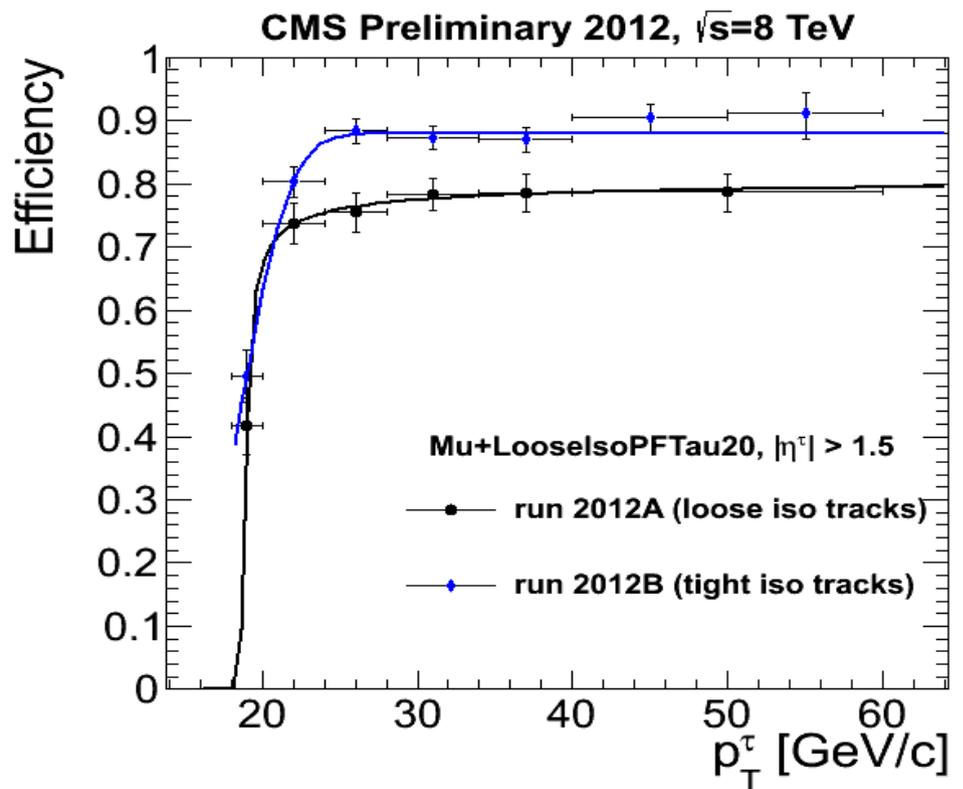
Efficiency measured using tag-and-probe technique with  $Z \rightarrow \tau^+ \tau^-$ ,  $\tau^- \rightarrow \mu + \tau\text{-hadr}$
