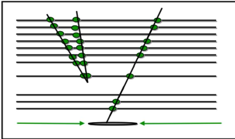
New collections of hits from the remaining clusters are created; pattern recognition is repeated, with looser constraints, in order to reconstruct **lower pT tracks** or **tracks with an associated vertex displaced from the beam-spot.**
