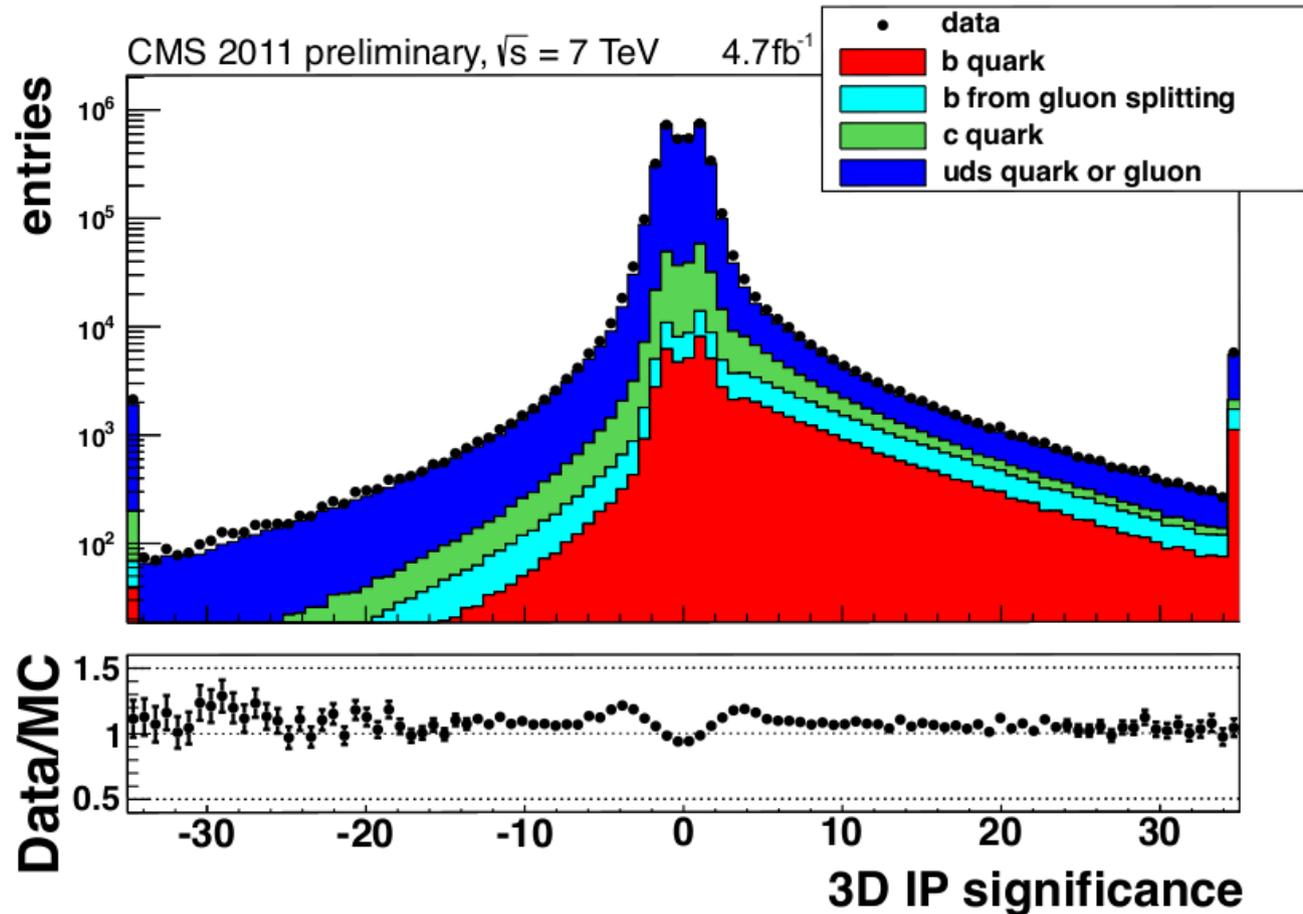
Excellent resolution in tracks and vertices reconstruction is used to build b-tagging discriminants, for example the Impact Parameter significance.
