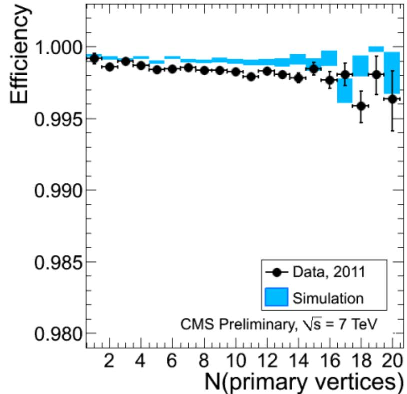
Tracking efficiency for muons measured in  $Z \rightarrow \mu\mu$  events, with a **tag and probe** technique.
