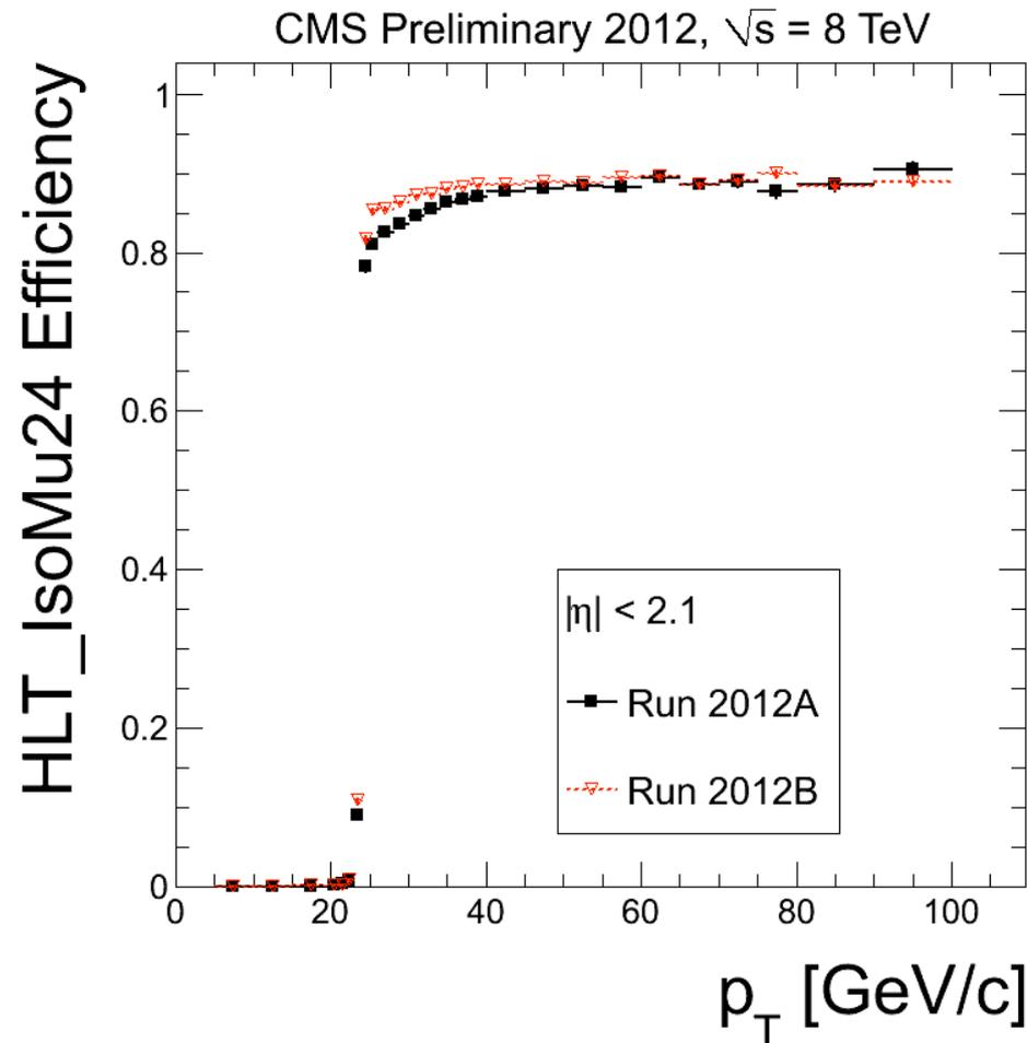
Muon triggers have very sharp turn-on curves, also thanks to tracking.
