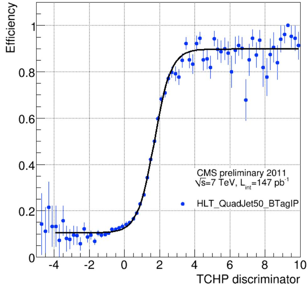
Turn-on curve of the HLT Track Counting High Purity (TCHP) discriminator efficiency, wrt offline. The TCHP discriminator is the significance of the third track (sorted by decreasing IP sign.). TCHP cut at 2 for this HLT path.
