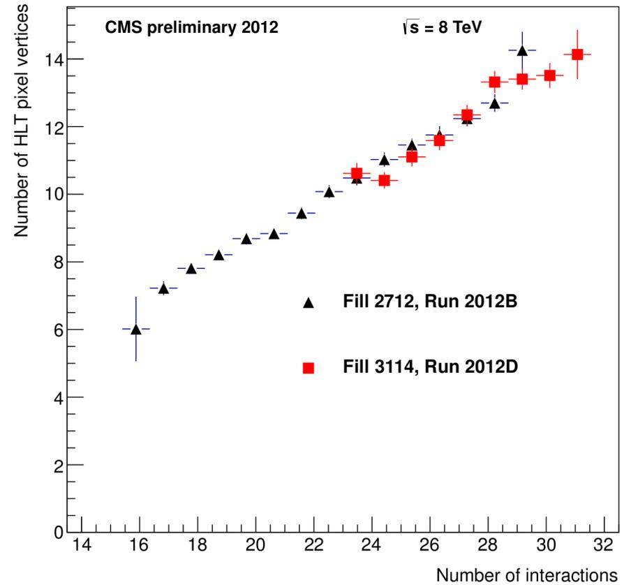
Number of interactions calculated from bunch luminosity measured with HF.
