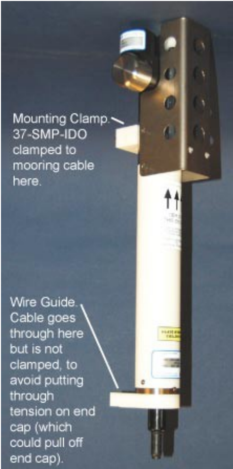
37-SMP-IDO shown; clamp and guide detail identical for 37-SIP-IDO
