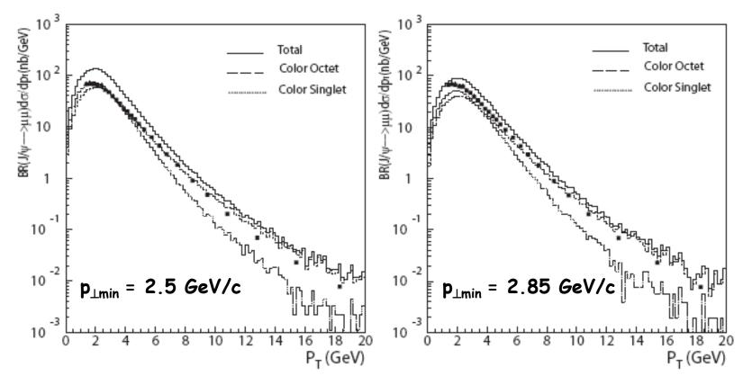
LHCb tuning of Pythia to fit the CDF measurements of  $J/\psi \rightarrow \mu + \mu - p_{\perp}$  differential cross section. CDF Collaboration, Phys. ReV. D71 032001, 2005 CSM and COM and leading order regularization  $p_{\perp min}$  cut-off tuned simultaneously. Matrix elements values (\*) extracted from: Nason P. et al. arXiv: hep-ph/0003142  $\langle Q\overline{Q} \left[ {}^{2S+1}L_{I}^{(C)} \right] \rangle$ (\*) 20
