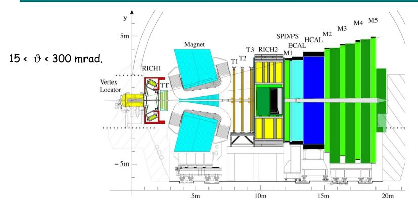
**VELO**: Silicon Strip detector for precise secondary vertex reconstruction. **TT,T1,T2,T2**: tracking stations, Silicon Strip and Straws to detect charged particles. **RICH1**, **RICH2**: Ring Imaging Cherenkov detectors for  $\pi/K/p$  separation. **ECAL**, **HCAL**: electromagnetic and hadronic calorimeters for trigger and energy flow. **M1-M5**: Muon stations for muon identication
